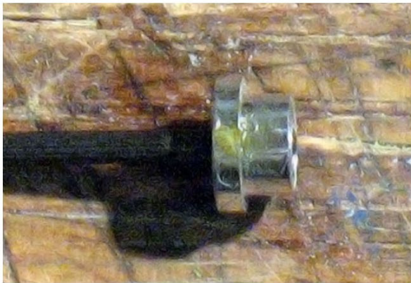
The rim pictured above shows a mold mark or burr. By sanding these spots smooth, you create a more rounded surface for tire to ride on.
