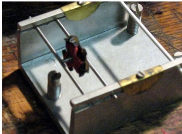
The armature pole pointing down is the heaviest and will have some material removed to balance the armature
