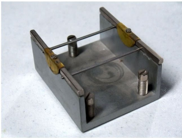
Here's a nice static balance jig I bought several years ago. You can build a similar jig to balance your armatures
