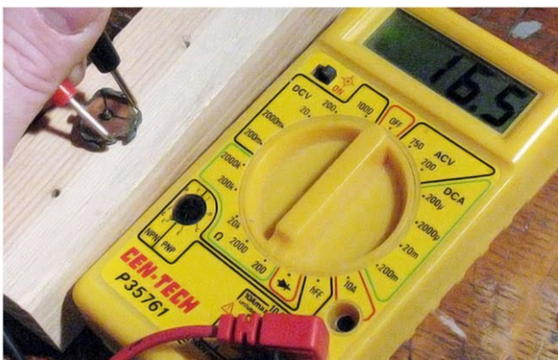
This is how to measure the Ohm rating of each armature pole
