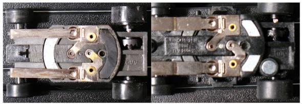
The left side image shows the motor magnets lowered flush with the bottom of the chassis. These are glued in place to keep them in this position. The right side image shows the Auto World X-Traction Ultra-G traction magnet lowered flush with the bottom of the chassis. It was .005" further up in the holder prior to this change.
