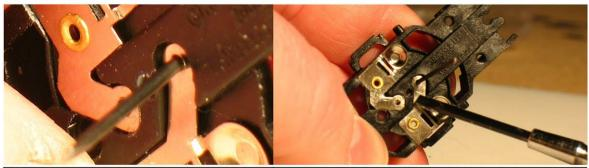
Here we can see the screwdriver we are using as our leverage point to flatten this brush cup tab.
