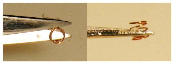
Sometimes the pick up shoe springs are too stiff or long or a combination of both and cause the shoes to bounce or bottom out on the chassis. If replacements are not available to sort through, I remove a single coil from the spring and stretch it very slightly. Place the cut side of the coil away from the pick up shoe (toward the chassis). The cut side can "thread" around the edge of the pick up shoe and come out.
