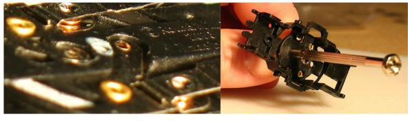
A bit difficult to see at this angle, but the brush cup tab on the right is bent inward toward the armature side of the chassis. This needs to be flattened to improve performance. We will insert a small rod, in this case a jeweler's screwdriver in the brush cup hole to use as leverage to straighten the brush cup tab.
