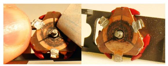
Clean the armature with some ultra-fine sanding film (1200 grit or finer) to polish the arm. You can also use erasers but make sure to wipe the residue from the comm. The residue does not conduct well and will hamper performance.
