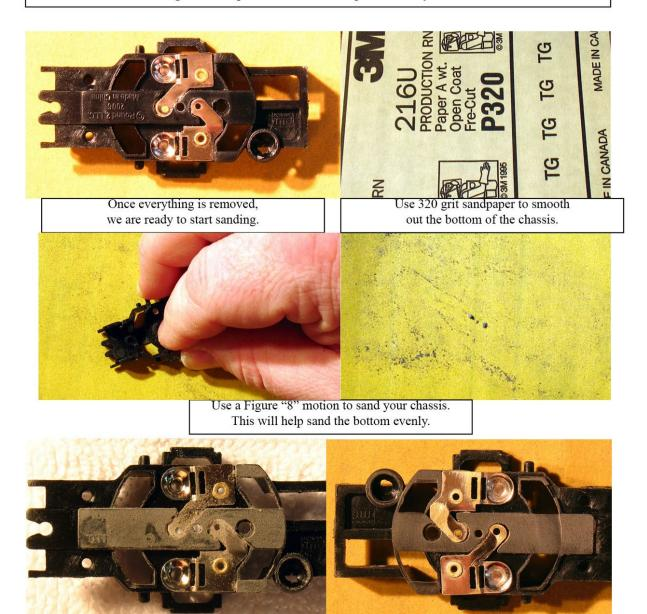
Remove material in small increments. You can't put material back once you sand it away. Check your progress frequently. The chassis on the left shows progress at about the half way point. The one on the right shows the finished job with all of the high spots removed.
