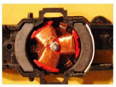
The pictures above show the sanding and shimming process to move the motor magnets closer to the armature. Take care to remove small amounts of plastic from the chassis and test fit frequently to make certain you do not remove too much material. The last picture on the right is the finished shim for that magnet.
