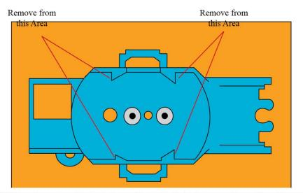
Take about .005" from the areas pointed out above. These tabs hold the magnet in position. Be careful not to remove too much, otherwise the magnet's face will contact the armature poles.
