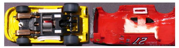
Left: Although this is an inline chassis, it shows how you can use double-sided foam tape to mount up a body to the chassis. Right: By using some scrap plastic, you can make snap in slots for the pancake chassis body mount tabs (See below). Either of these methods will allow you to mount the bodies lower, dropping the center of gravity and improving handling characteristics.
