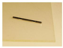
Here is a rear axle placed on a piece of glass. The smooth and level surface of the glass will easily show any bends or abnormalities with the axle. A mirror can be used for the process as well. This one is straight and is ready to go back on the chassis.
