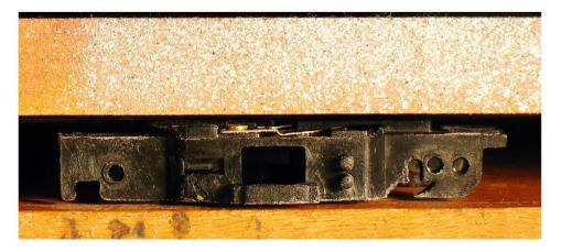
Here is a chassis clamped up for straightening. I use this method whether I'm using hot water or the heat gun to warm up the chassis material for the straightening process. This same clamp is used on the gear plate, once the gears and armature are removed. There are some manufactured jigs that force the chassis straight with rods running through the axle holes. These types of jigs also help align the axles as well as straightening the chassis.
