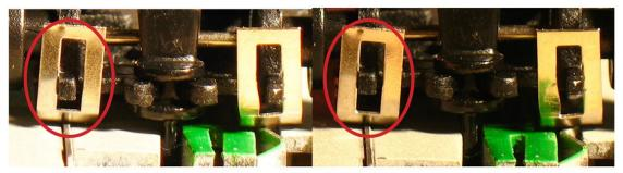
On the left we have a set of pick up shoes that are bottomed out. So if it hits any high or low rail it is going to jar the chassis, most likely out of the slot. On the right we have a shorter spring with a tiny bit of extra tension, but soft and springy. This leaves a little play in the pick up shoe travel. Think of this as a suspension point on the chassis. Always keep contact with the rails, but with enough play to absorb the slot car equivalent of a potholes.
