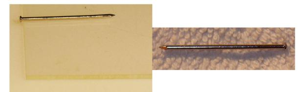
The front axle on the left, sitting on the glass, is slightly bent. This is easily seen when rolling the axle across the glass. This is not something that can repaired easily and should be replaced. The axle on the right is a new, straight component. It's a good practice to roll test new axles on a glass surface, just to make sure they are straight.
