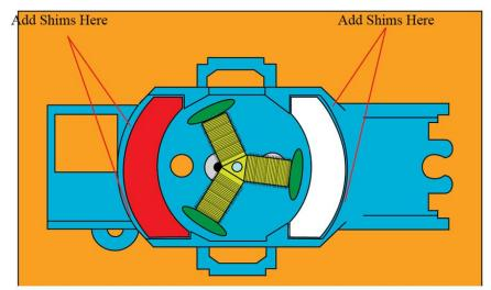
Push the shim material in behind the magnets in the locations pointed out above. Make this a nice tight fit without distorting the chassis. The closer you get the magnets to the armature, the greater the torque you can generate.
